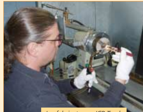
Jay fabricates an ICP Torch.
